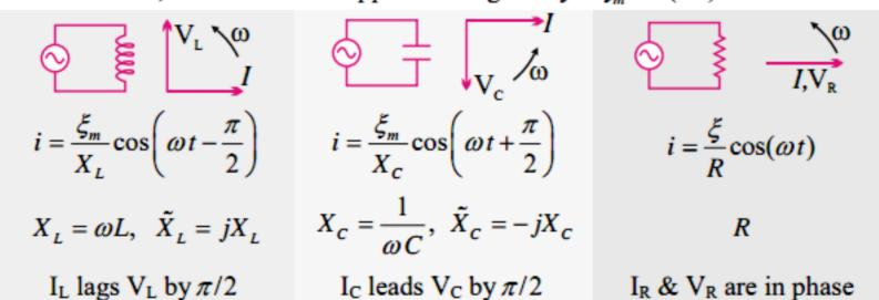
LCR series circuit: LIC: Read clockwise; but we take anticlockwise positive Note: In diagram below,  $V_L$ ,  $V_C$  &  $V_R$  are all peak values.
