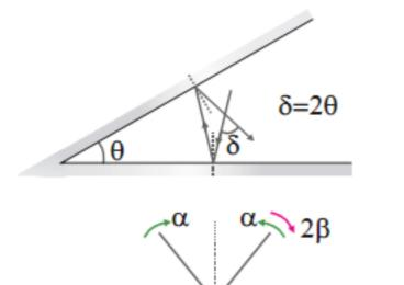
Deviation is angle between incident ray and reflected/refracted ray.
