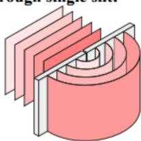
The widths of the slits must be of the same order as the wavelength of the light.
