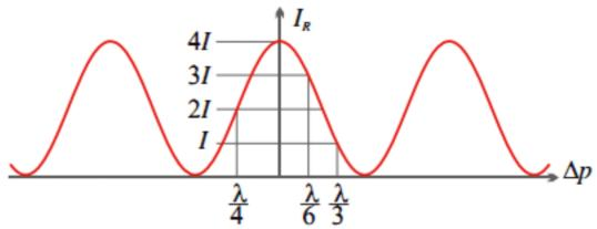
When  $d \sim \lambda$ , then the number of fringes formed in finite distance are 9. And we can see that intensity of nearby maximas do not remain constant.
