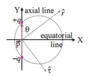
Torque on a pure dipole in a uniform Electric field:  $\vec{\tau} = \vec{p} \times \vec{E}$
