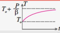
Rate of gain of heat =  $P - \sigma A \left[ T^4 - T_o^4 \right]$
