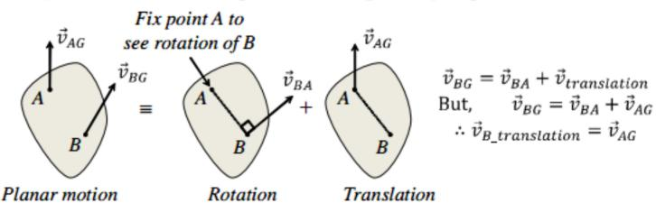
If we analyze w.r.t. COM, we can say that:  $\vec{v}_{BG} = \vec{v}_{CG} + \vec{\omega} \times \vec{r}_{BC}$
