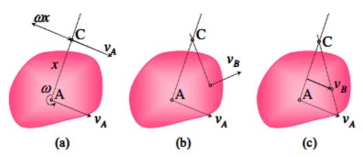
Constraint equation: Written at contact points where no slipping (sliding) takes place and that can also be thought as pure rolling.
