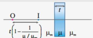
Apparent shift =  $t \left( 1 - \frac{1}{\mu_r} \right)$  is always in the direction of incident light
