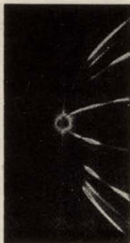
FIG. 42.23. Mass Spectrometer. Positive-ray parabolas due to mercury, carbon monoxide, oxygen and carbon ions.
