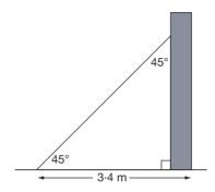
A prop in the form of an isosceles triangle constructed out of timber is placed against a vertical wall. If the length of the side along the horizontal ground is 3.4 m the length of the hypotenuse to 2 dp is obtained as follows:
