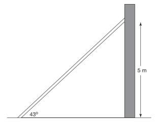
To strengthen a vertical wall a strut has to be placed 5 m up the wall and inclined at an angle of  $43^{\circ}$  to the ground. To do this the length of the strut must be ......
