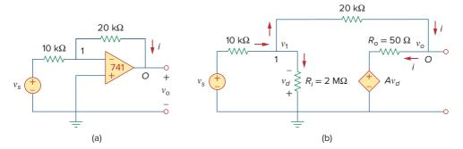
**Figure 5.6** For Example 5.1: (a) original circuit, (b) the equivalent circuit.
