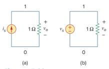
**Figure 17.33** Fourier analysis with *PSpice* using: (a) a current source, (b) a voltage source.
