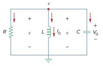
**Figure 8.13** A source-free parallel *RLC* circuit.
