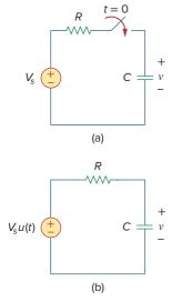
**Figure 7.40** An *RC* circuit with voltage step input.
