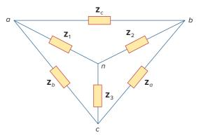
**Figure 9.22** Superimposed *Y* and  $\Delta$  networks.
