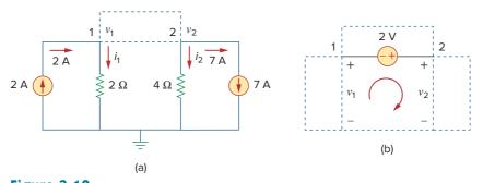
**Figure 3.10** Applying: (a) KCL to the supernode, (b) KVL to the loop.
