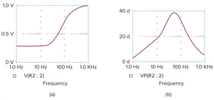
**Figure 14.54**For Practice Problem 14.15: (a) magnitude plot, (b) phase plot of the frequency response.
