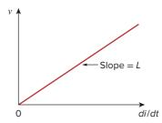
**Figure 6.24** Voltage-current relationship of an inductor.
