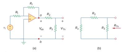
**Figure 7.60** Obtaining  $V_{\text{Th}}$  and  $R_{\text{Th}}$  across the capacitor in Fig. 7.59.
