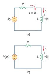
**Figure 7.48** An *RL* circuit with a step input voltage.
