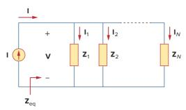
**Figure 9.20** *N* impedances in parallel.
