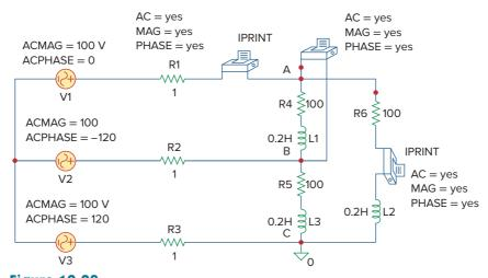
**Figure 12.28** Schematic for the circuit in Fig. 12.27.
