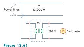
A transformer providing isolation between the power lines and the voltmeter.
