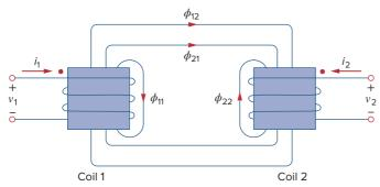
**Figure 13.4** Illustration of the dot convention.
