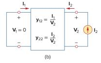
**Figure 19.12** Determination of the *y* parameters: (a) finding  $y_{11}$  and  $y_{21}$ , (b) finding  $y_{12}$
