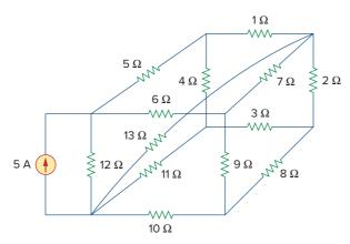
**Figure 3.16** A nonplanar circuit.
