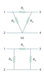
**Figure 2.48** Two forms of the same network: (a)  $\Delta$ , (b)  $\Pi$ .
