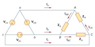
**Figure 12.17** A balanced  $\Delta$ - $\Delta$  connection.
