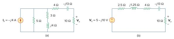
**Figure 10.18** Solution of the circuit in Fig. 10.17.
