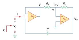
**Figure 10.41** Capacitance multiplier.
