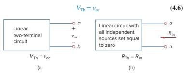
**Figure 4.24** Finding  $V_{\text{Th}}$  and  $R_{\text{Th}}$ .
