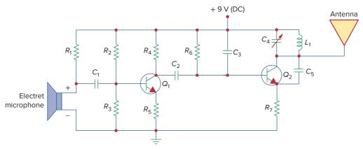
**Figure 1.2** Electric circuit of a radio transmitter.
