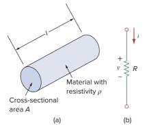
**Figure 2.1**(a) Resistor, (b) Circuit symbol for resistance.
