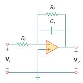
**Figure 14.42** Active first-order low-pass filter.
