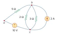
**Figure 2.11** The three-node circuit of Fig. 2.10 is redrawn.
