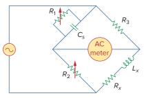
**Figure 9.84** Maxwell bridge; For Prob. 9.84.
