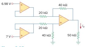
**Figure 5.27** Instrumentation amplifier; for Practice Prob. 5.8.
