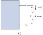
Figure 2.2 (a) Short circuit (R = 0), (b) Open circuit  $(R = \infty)$ .
