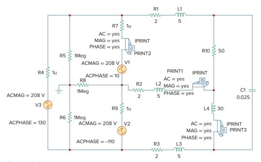
**Figure 12.31** Schematic for the circuit in Fig. 12.30.
