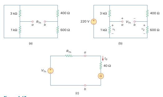
**Figure 4.65** For Example 4.18: (a) Finding  $R_{Th}$ , (b) finding  $V_{Th}$ , (c) determining the current through the galvanometer.
