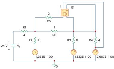
**Figure 3.35** The schematic of the circuit in Fig. 3.34.
