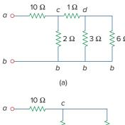
**Figure 2.38** Equivalent circuits for Example 2.10.
