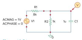
**Figure 14.51** The schematic for the circuit in Fig. 14.50.
