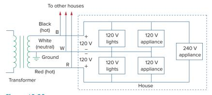
**Figure 12.38**Single-phase three-wire residential wiring.
