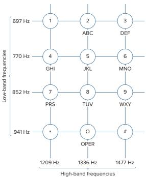
**Figure 14.64** Frequency assignments for touch-tone dialing.
