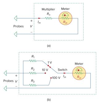
**Figure 2.60**Voltmeters: (a) single-range type, (b) multiple-range type.
