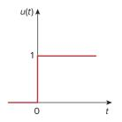
**Figure 7.23** The unit step function.
