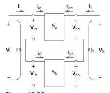
**Figure 19.39** Series connection of two two-port networks.
