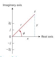
**Figure 9.6** Representation of a complex number  $z = x + jy = r/\phi$ .
