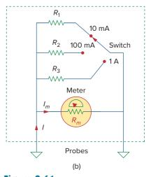
**Figure 2.61**Ammeters: (a) single-range type, (b) multiple-range type.
