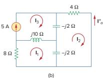
Figure 10.12 Solution of Example 10.5.
