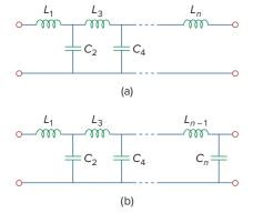
**Figure 19.61** *LC* ladder networks for low-pass filters of: (a) odd order, (b) even order.
