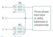
**Figure 12.34**Two-wattmeter method for measuring three-phase power.
