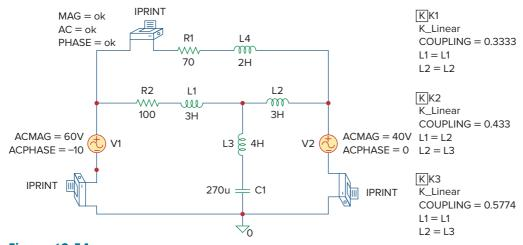
**Figure 13.54** Schematic of the circuit of Fig. 13.53.
