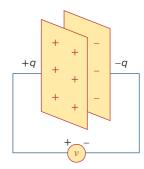
**Figure 6.2** A capacitor with applied voltage v.
