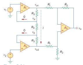
**Figure 5.26** Instrumentation amplifier; for Example 5.8.
