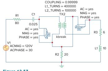
**Figure 13.57** The schematic for the circuit in Fig. 13.56.
