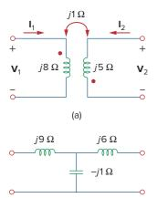
**Figure 13.28** For Example 13.6: (a) circuit for coupled coils of Fig. 13.27, (b) T-equivalent circuit.
