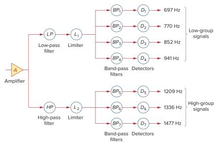
**Figure 14.65**Block diagram of detection scheme.
