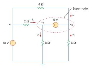
**Figure 3.7** A circuit with a supernode.
