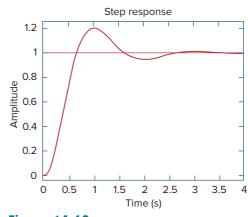
Figure 14.60 The Step response of  $H(s) = 12/(s^2 + 3s + 12)$ .
