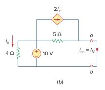
Figure 4.44 For Example 4.12: (a) finding  $R_N$ , (b) finding  $I_N$ .
