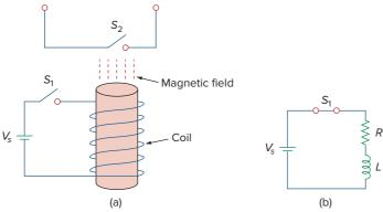
**Figure 7.77** A relay circuit.
