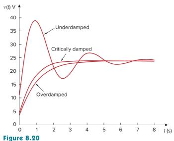
For Example 8.7: response for three degrees of damping.
