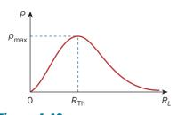
**Figure 4.49** Power delivered to the load as a function of  $R_L$ .
