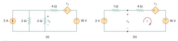
**Figure 4.21** For Example 4.7: Applying source transformation to the circuit in Fig. 4.20.
