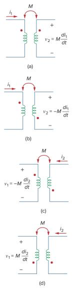
**Figure 13.5** Examples illustrating how to apply the dot convention.
