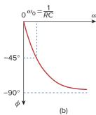
**Figure 14.3** Frequency response of the *RC* circuit: (a) amplitude response, (b) phase response.
