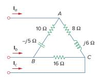
**Figure 12.24** Unbalanced Δ-load; for Practice Prob. 12.9.
