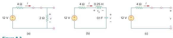
**Figure 8.3** Equivalent circuit of that in Fig. 8.2 for: (a)  $t = 0^-$ , (b)  $t = 0^+$ , (c)  $t \to \infty$ .
