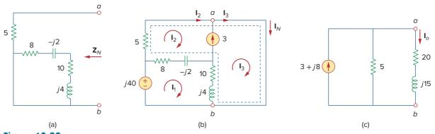
Figure 10.29 Solution of the circuit in Fig. 10.28: (a) finding  $\mathbf{Z}_N$ , (b) finding  $\mathbf{V}_N$ , (c) calculating  $\mathbf{I}_O$ .
