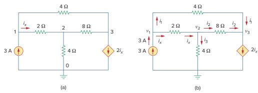
**Figure 3.5** For Example 3.2: (a) original circuit, (b) circuit for analysis.
