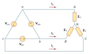
Figure 12.18 A balanced  $\Delta$ -Y connection.
