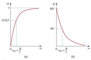
**Figure 14.5** Frequency response of the *RL* circuit in Fig. 14.4.
