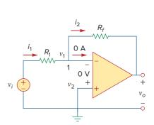
**Figure 5.10**The inverting amplifier.
