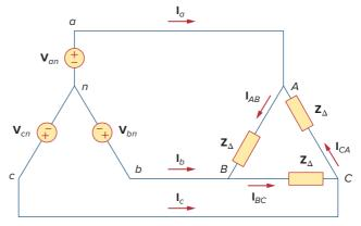
**Figure 12.14** Balanced Y-Δ connection.
