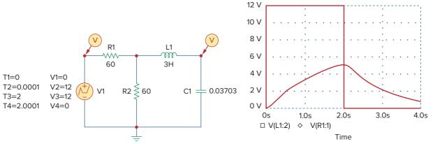
**Figure 8.36** Schematic for the circuit in Fig. 8.35(b).
