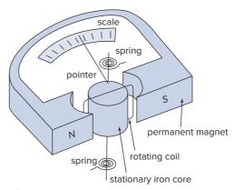
**Figure 2.58** A d'Arsonval meter movement.
