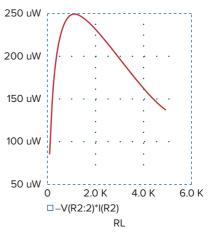
**Figure 4.57** For Example 4.15: the plot of power across  $R_L$ .
