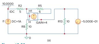
**Figure 19.50** For Example 19.15: (a) computing  $\mathbf{h}_{11}$  and  $\mathbf{h}_{21}$ , (b) computing  $\mathbf{h}_{12}$  and  $\mathbf{h}_{22}$ .
