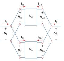
**Figure 19.40** Parallel connection of two two-port networks.
