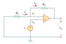
**Figure 5.16**The noninverting amplifier.
