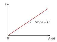
**Figure 6.6**Current-voltage relationship of a capacitor.
