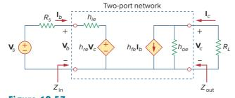
**Figure 19.57**Transistor amplifier with source and load resistance.
