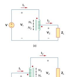
**Figure 13.42**(a) Step-down autotransformer, (b) step-up autotransformer.
