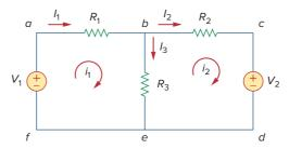
**Figure 3.17** A circuit with two meshes.
