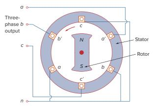
**Figure 12.4** A three-phase generator.
