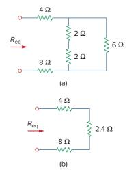
**Figure 2.35** Equivalent circuits for Example 2.9.
