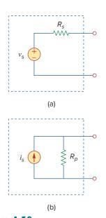
**Figure 4.58**(a) Practical voltage source, (b) practical current source.
