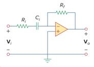
**Figure 14.43** Active first-order high-pass filter.
