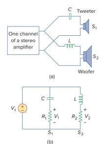
**Figure 14.66**(a) A crossover network for two loudspeakers, (b) equivalent model.
