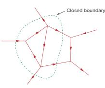
**Figure 2.17** Applying KCL to a closed boundary.
