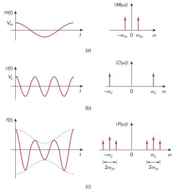
**Figure 18.22** Time domain and frequency display of: (a) modulating signal, (b) carrier signal, (c) AM signal.
