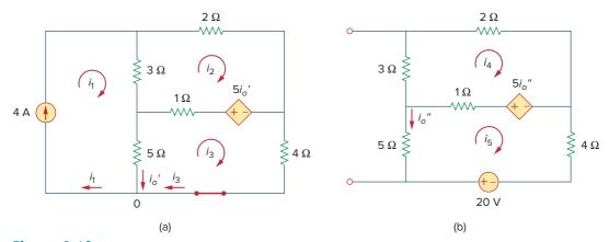
**Figure 4.10** For Example 4.4: Applying superposition to (a) obtain  $i'_{o}$ , (b) obtain  $i''_{o}$ .
