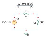
**Figure 4.56** Schematic for the circuit in Fig. 4.55.
