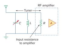
**Figure 14.63** The tuner circuit for Example 14.17.
