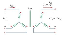
**Figure 13.46** Y-Y three-phase transformer connection.
