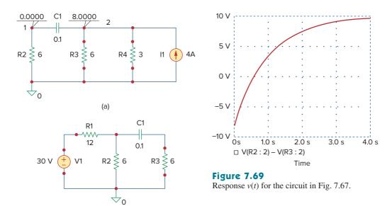
**Figure 7.68** (a) Schematic for dc analysis to get v(0), (b) schematic for transient analysis used in getting the response v(t).
