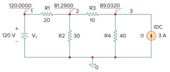
**Figure 3.32** For Example 3.10; the schematic of the circuit in Fig. 3.31.
