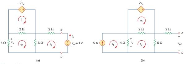
**Figure 4.32** Finding  $R_{\text{Th}}$  and  $V_{\text{Th}}$  for Example 4.9.
