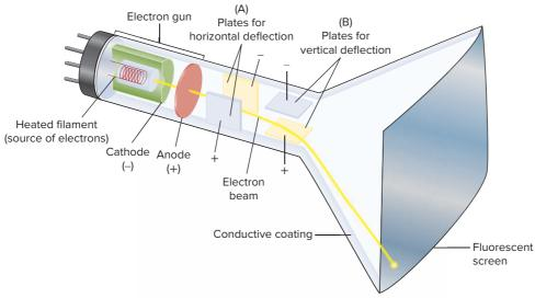
Figure 1.17 Cathode-ray tube.
