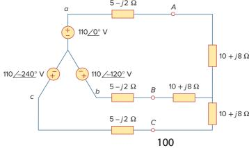
**Figure 12.13**Three-wire Y-Y system; for Example 12.2.
