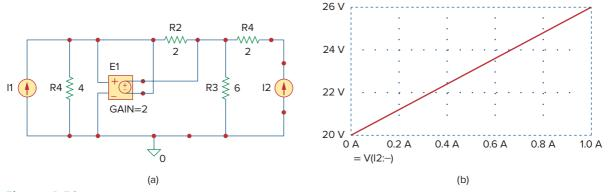
**Figure 4.53** For Example 4.14: (a) schematic and (b) plot for finding  $R_{\text{Th}}$  and  $V_{\text{Th}}$ .
