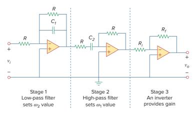
**Figure 14.45** Active band-pass filter.
