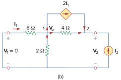
**Figure 19.18** Solution of Example 19.4: (a) finding  $y_{11}$  and  $y_{21}$ , (b) finding  $y_{12}$  and  $y_{22}$ .
