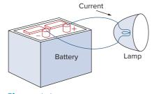
**Figure 1.1** A simple electric circuit.
