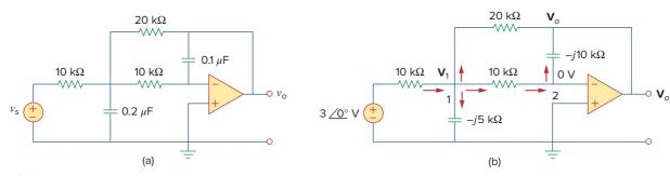
**Figure 10.31** For Example 10.11: (a) the original circuit in the time domain, (b) its frequency domain equivalent.
