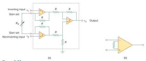
**Figure 5.38**(a) The instrumentation amplifier with an external resistance to adjust the gain, (b) schematic diagram.
