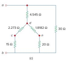
**Figure 2.53** Equivalent circuits to Fig. 2.52, with the voltage source removed.
