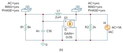
**Figure 19.53** For Example 19.16: (a) circuit for determining  $\mathbf{z}_{11}$  and  $\mathbf{z}_{21}$ , (b) circuit for determining  $\mathbf{z}_{12}$  and  $\mathbf{z}_{22}$ .
