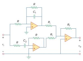
**Figure 14.47** Active band-reject filter.
