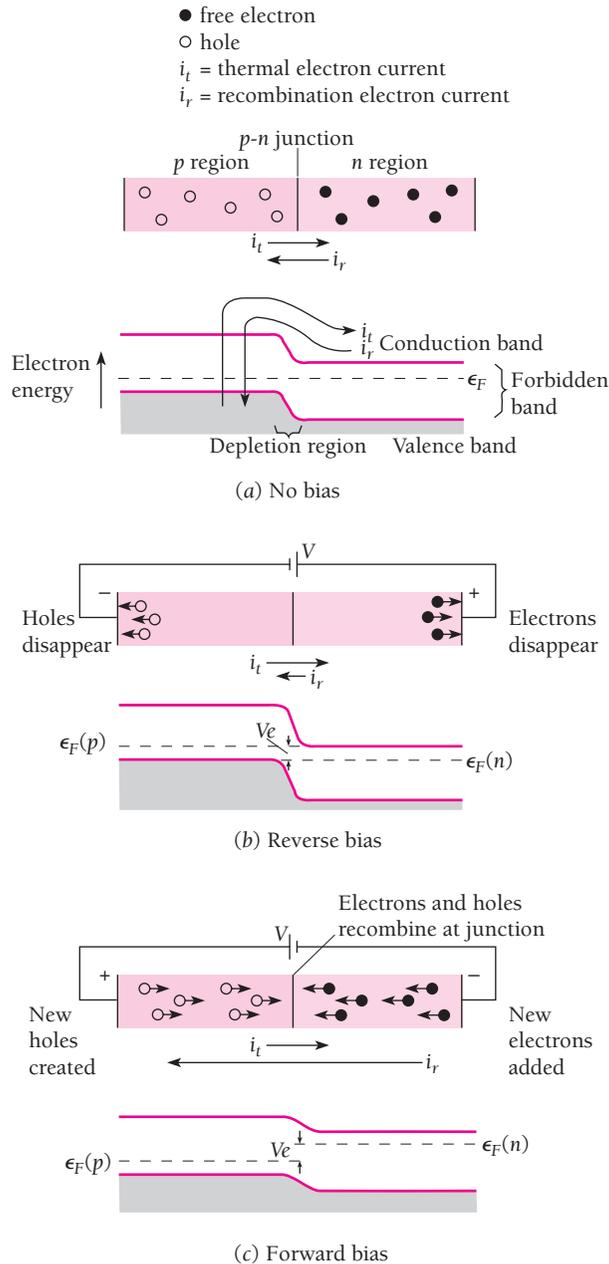
Figure 10.30 Operation of a semiconductor diode.
