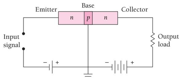
Figure 10.36 A simple junction-transistor amplifier.
