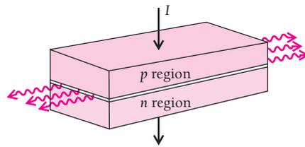
**Figure 10.32** A semiconductor laser. Each dimension is less than a millimeter and its light output, as in all lasers, is coherent. The junction between the  $p$  and  $n$  regions from which the light emerges is only a few micrometers thick.
