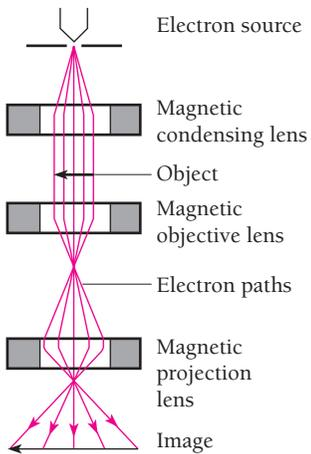
**Figure 3.5** Because the wavelengths of the fast electrons in an electron microscope are shorter than those of the light waves in an optical microscope, the electron microscope can produce sharp images at higher magnifications. The electron beam in an electron microscope is focused by magnetic fields.
