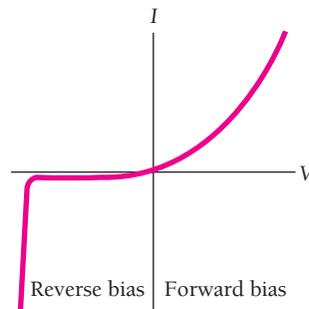
**Figure 10.35** Voltage-current characteristic of a Zener diode.
