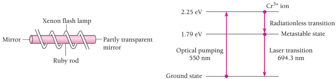
Figure 4.27 The ruby laser. In order for stimulated emission to exceed stimulated absorption, more than half the  $\text{Cr}^{3+}$  ions in the ruby rod must be in the metastable state. This laser produces a pulse of red light after each flash of the lamp.
