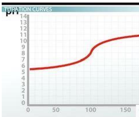
Titration curve for weak acid vs weak base
